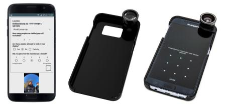
Fig. 2. The rating application (left) and the smartphone enclosure including, fish-eye lens (center: rendered design, right: prototype).
