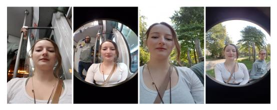
Fig. 3. Different fields of view of a mobile phone enclosure using a fish-eye lens, extending the front facing camera. Two staged situations in a train (left) and in a park (right).
