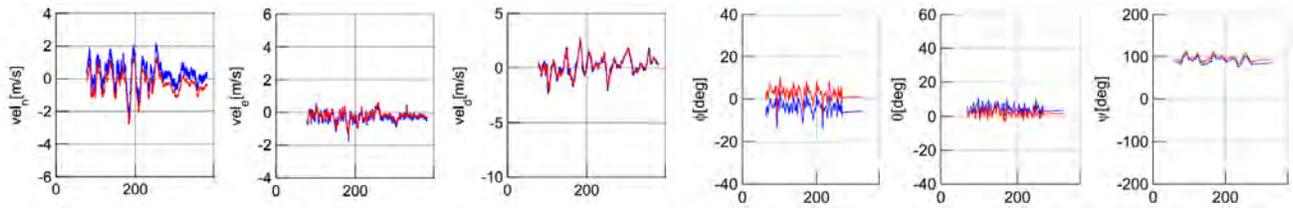
Figure 5: Velocity data and Euler angles of the copter during the first task (i.e., hovering). Since the copter has two build in processors (Gumstix: red – FPGA: blue) reading the velocity sensor, we have two data values for each velocity and Euler angle.
