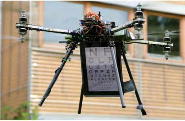
Figure 4: Midair display prototype with Snellen chart.
