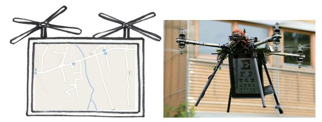
Figure 2: A sketch of the envisioned copter display (left) and the actual prototype (right).
