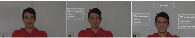
Figure 1: AR devices allow dynamic information overlays. Gaze provides a mean to select information on demand when the user looks at that particular information. This allows the user to keep the UI uncluttered (a), but at anytime make specific information appear (b). Without gaze, showing all information can distract the user (c)
