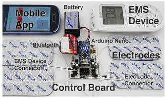
Figure 3. The hardware prototype including the EMS device, self-adhesive pads, the wireless control board, and a mobile device with control apps.
