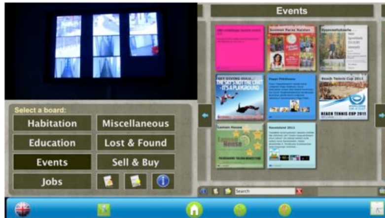
Fig. 10 – Digifieds user interface: The display client shows an overview of the different views on the left, the active view, containing the actual digifieds, on the right.
