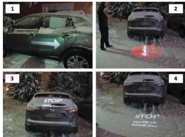
Figure 1. Car external surface display concepts included in the focus group study. The displays are created using a handheld projector. 1) Navigation guidance for pedestrians or other (car) drivers 2) Warning for pedestrians/other car drivers of car reversing. 3&4) Warning for pedestrians or other car drivers of other vehicles moving.
