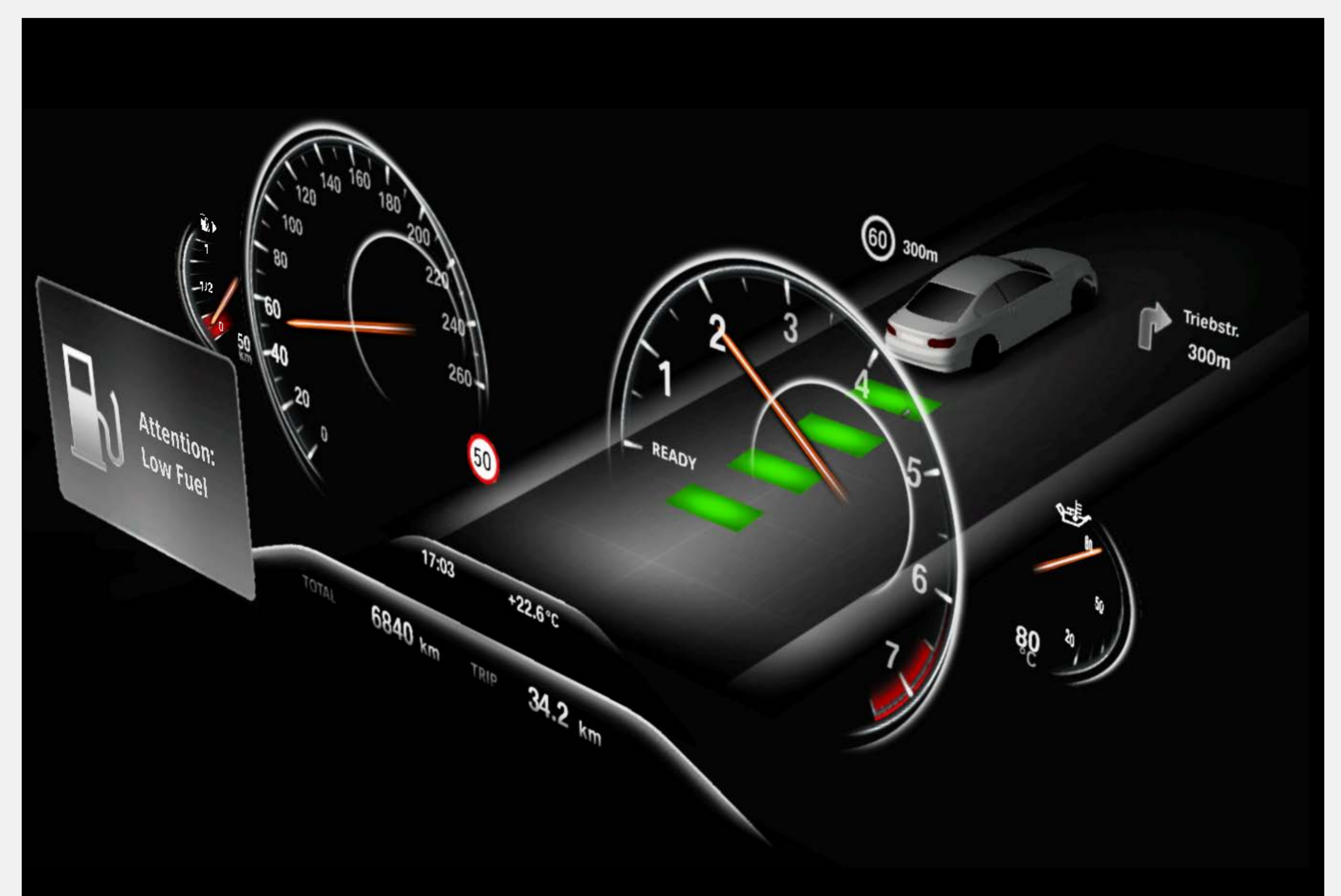
Side view of the instrument cluster showing the depth layout of the UI elements.
